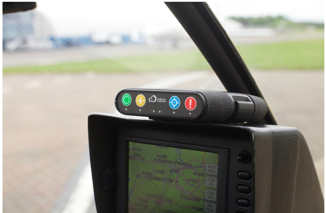
If you are unable to position the RockAIR anywhere with such a view, you should consider installing an external antenna or antennae. This is typically a dual mode GPS/Iridium antenna and a separate cellular antenna. This requires notification at time of purchase, or a return to your distributor for an approved modification.
