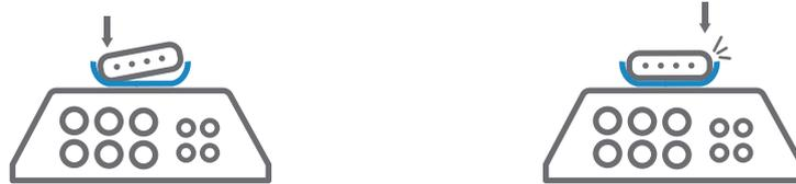
To remove the RockAIR from the mounting clip, move the top of the right side of the clip away from the RockAIR and lift the RockAIR clear.
