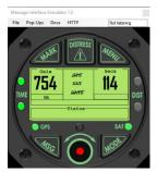
The default home screen shows hopper quantity and a countdown indicating the time in seconds until the next tracking interval. The tracking <u>mode</u> can be changed by clicking the "Mode" button. The LED illumination and the Tracker Box title will change accordingly, If the tracking mode is set to time, the Status window will show a brief message when the event is transmitted.
