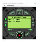
The pilot can view the raw latitude and longitude data if, for example, they wish to enter it into the aircraft GPS. To do this, rotate the Selector Knob.
