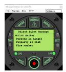
Outbound messaging is used to enable the pilot to "Mark" the position of a location of interest. This point will then be displayed along with the tracking data on the Tracplus map. The list of messages is configurable.
