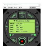
The MI also shows COM and TXT data associated with the task. To move between the NAV, COM and TXT screens, press the Selector Knob.
