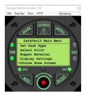
The menu system enables a variety of DataVault parameters to be adjusted. (The simulator illustrates the screens used to control the parameters, but some of the parameters themselves cannot be adjusted.)
