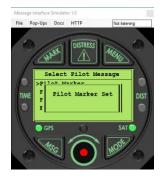
A pop-up window appears to confirm the despatch of the message. This example shows a "Pilot Marker" message, which also stores the location in the Waypoint list.
