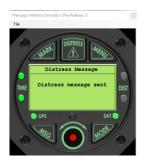
To send a distress message, the Distress key should be pressed twice. The display will show that a message has been sent. These messages are acknowledged automatically by the TracPlus service. When the acknowledgement is received, the display will indicate accordingly.
