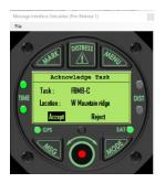
The MI indicates immediately that a task message has arrived. The pilot can accept or reject the message by rotating the Selector Knob and clicking the appropriate response.
