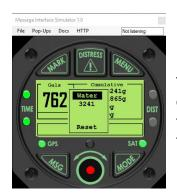
The "Hppr/Cumulative" screen shows the total quantity of fluid dropped by type. To reset this total, press Selector Knob, rotate it to select the type of fluid, then press the Selector Knob twice.
