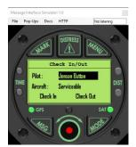
To change the pilot or the status, use the Selector Knob to highlight the required item, then click. The display will change to indicate that the item has been selected for adjustment and the Selector Knob can be used to change the information. When the pilot name is correct, click to select it.
