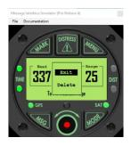
The pilot can return to the home screen by pressing MSG at any time. Alternatively, press Menu and select Exit from the pop-up screen which appears.
